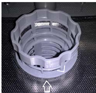
Poorly secured filter
